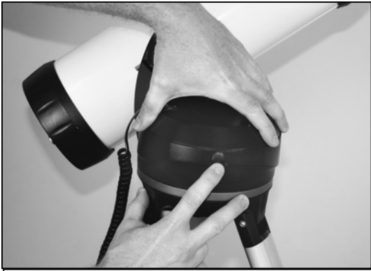
Figure 2-9 – Removing the Battery Compartment Lid
