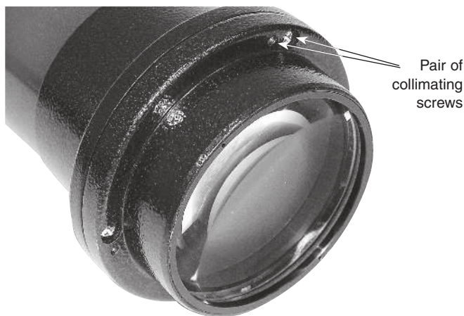
Figure 6-2. The lens cell of the StarSeeker 100. There are three pairs of collimating screws; each pair of screws work together to adjust the tilt of the lens.
