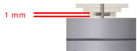
Pic. 12: Mounting the pulley
