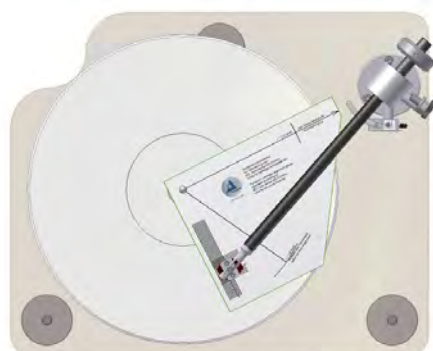
Pic. 10: Alignment of the cartridge
