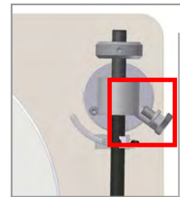
Illustration 3 : Maximum antiskating (Screw is screwed in)
