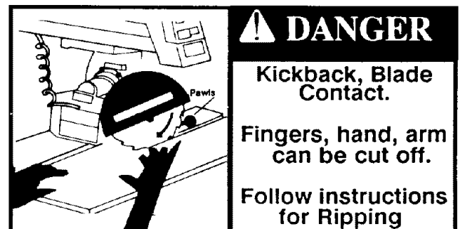
Fig. 3 Blade Contact Safety Sign
