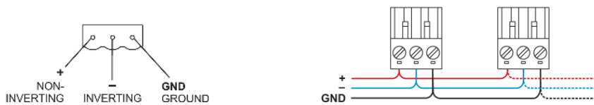
Figure 8. Balanced analogue input pin-out (left) and daisy-chaining cables in the analogue input Euroblock connector (right).
