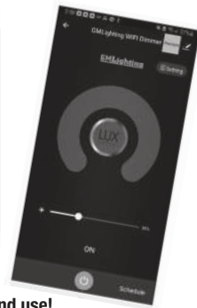
4. During Auto Scan, cycle dimmer On/Off 3 times. Dimmer will be recognized.
