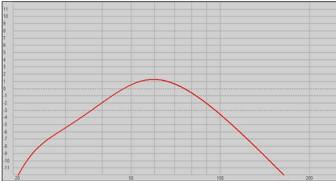
Frequenzgang mit Tiefpass-Filter @ 80 Hz / 12 dB/Okt frequency response with low pass filter @ 80 Hz / 12 dB/oct
