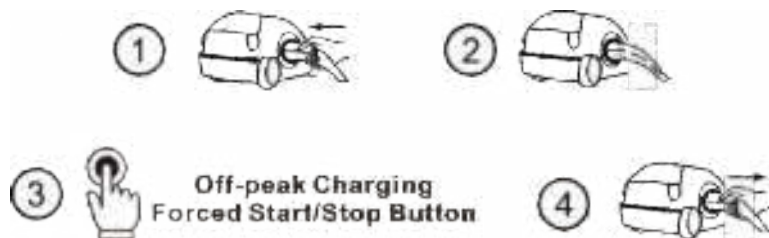
Plug&Charge mode operation process flow
