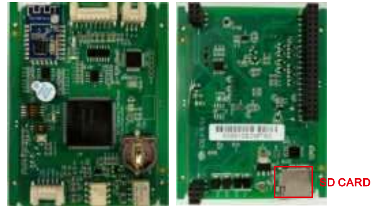
Micro SD slot of 22kW charger
