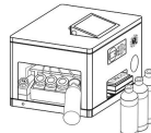
Add ink into ink container according the color labels on the top of the cap
