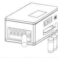
Add ink into ink container according the color labels on the top of the cap
