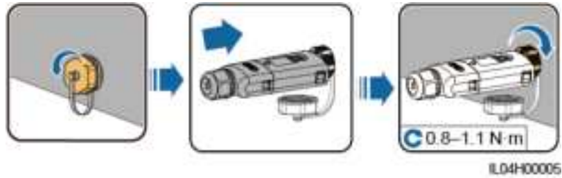
Figure 5-36 Installing a WLAN-FE Smart Dongle (WLAN communication)
