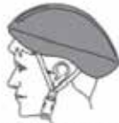
INCORRECT FITTING – FOREHEAD IS EXPOSED AND VULNERABLE TO SERIOUS INJURY.
