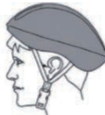
INCORRECT FITTING – FOREHEAD IS EXPOSED AND VULNERABLE TO SERIOUS INJURY.
