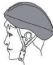
INCORRECT FITTING – FOREHEAD IS EXPOSED AND VULNERABLE TO SERIOUS INJURY.
