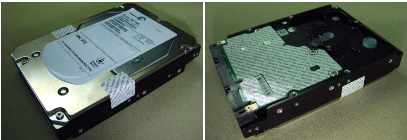
Figure 11. Example of FIPS tamper evidence labels.
