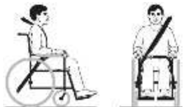
Figure 3b - Proper routing and positioning of belt restraints on the wheelchair occupant.
