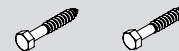
Two (2) 1/2" hex head lag bolt 1 1/2" (38 mm) long or equivalent hardware to secure the unit heater installation bracket.
