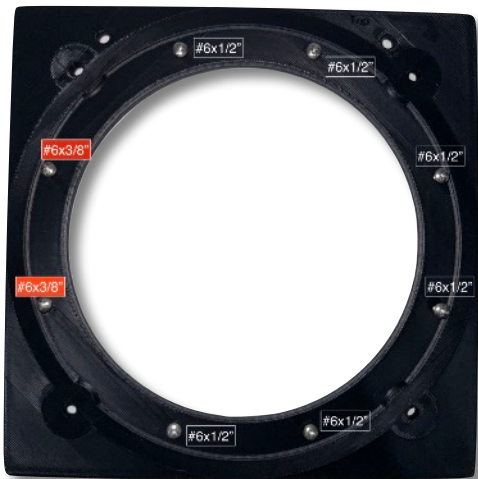
Screws glued to condenser/fan adapter plate
