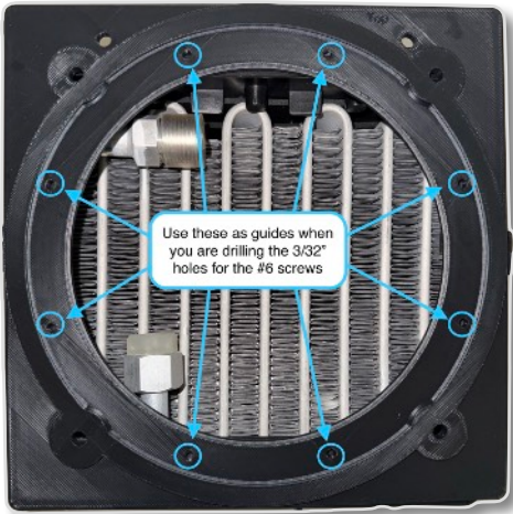
Drilling holes in the condenser housing
