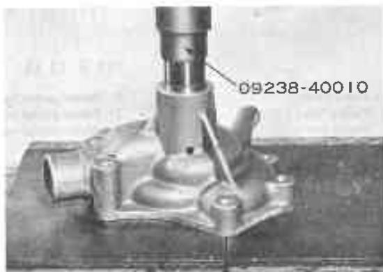
Fig. 7-7 Installing Bearing V3197
