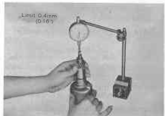
Fig. 10-12 Checking Thrust Clearance
