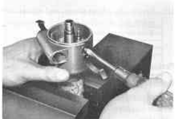
Fig. 10-21 Installing Cap Springs V3685
