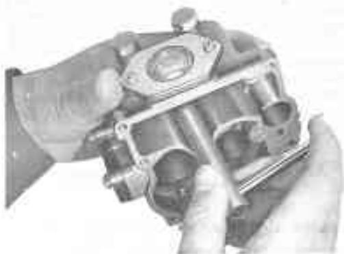
Fig. 5-60 Power Valve Removal B0113
