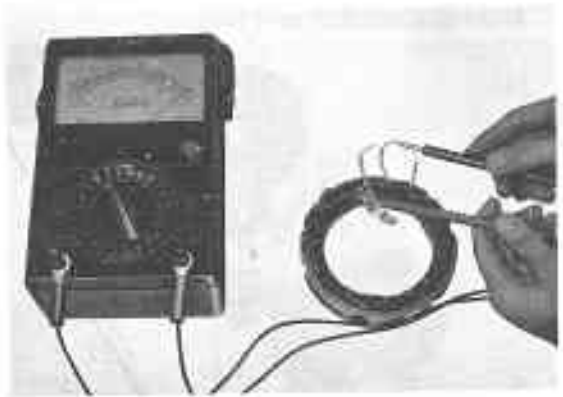
Fig. 8-17 Testing Stator Coil for Open Circuit
