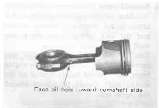
Fig. 3-57 Assembling Piston & Connecting Rod
