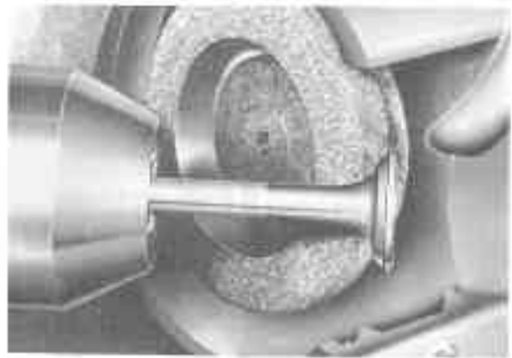
Fig. 3-21 Grinding Valve V0716
