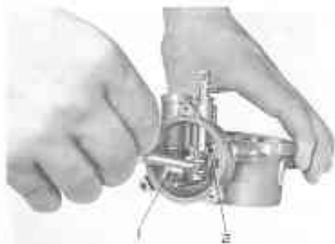
Fig. 5-37 Sliding Rod Removal V3999
