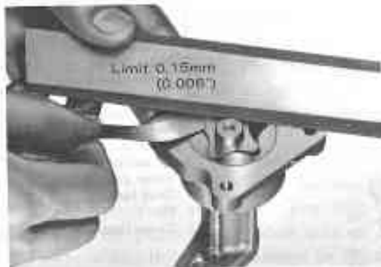
Fig. 6-6 Checking Side Clearance V3190
