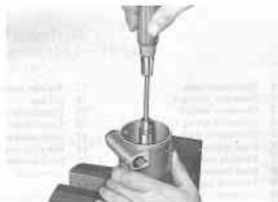
Fig. 10-9 Removing Distributor Cam V3678
