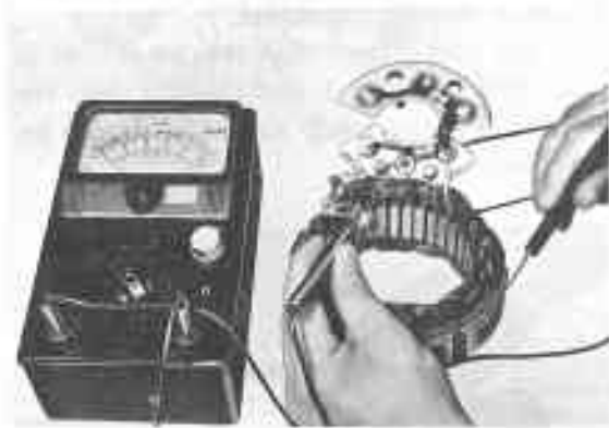
Fig. 8-15 Testing Stator Coil for Insulation
