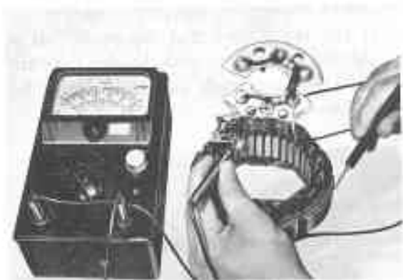
Fig. 8-15 Testing Stator Coil for Insulation B0041
