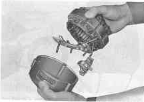
Fig. 8-11 Stator with Rectifier Holder Removal
