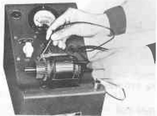
Fig. 9-10 Testing Armature Coil for Ground
