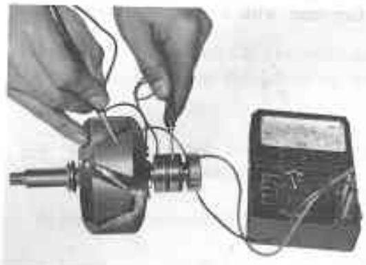
Fig. 8-14 Testing Rotor Coil for Ground V2197
