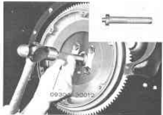
Fig. 3-70 Installing Bearing B1011 V4700
