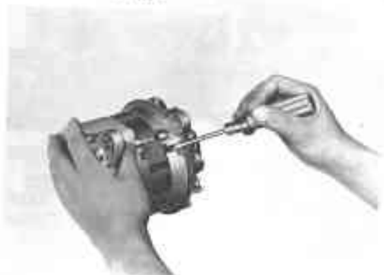
Fig. 8-7 Drive End Frame Removal
