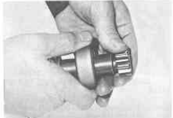
Fig. 9-21 Checking Starter Clutch VI817
