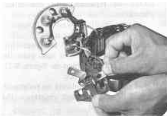
Fig. 8-22 Assembling Brush Holder B0043
