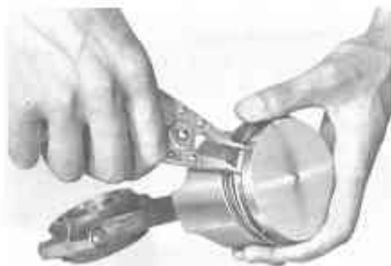
Fig. 3-11 Piston Ring Removal V3127
