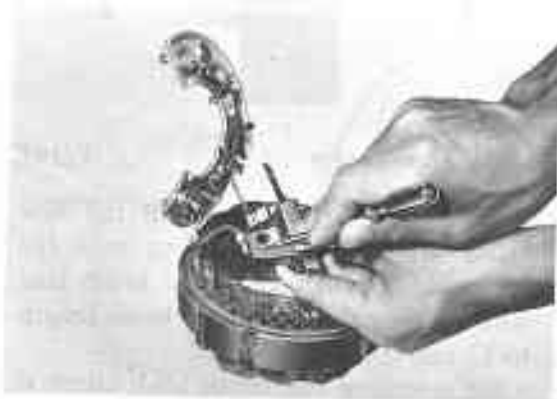
Fig. 8-12 Brush Holder Removal
