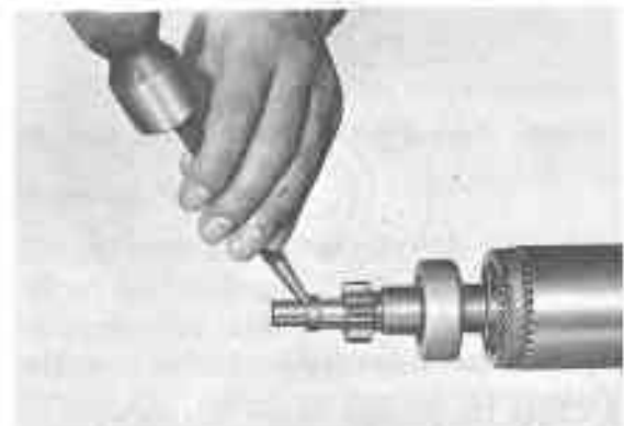
Fig. 9-22 Calking Stopper Collar B0037
