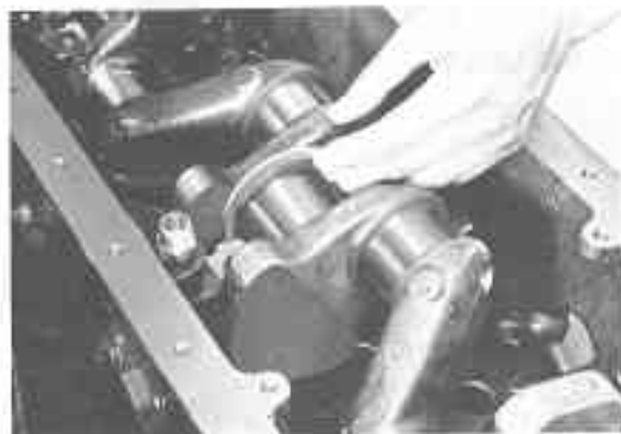
Fig. 3-62 Inserting Thrust Washer V3182
