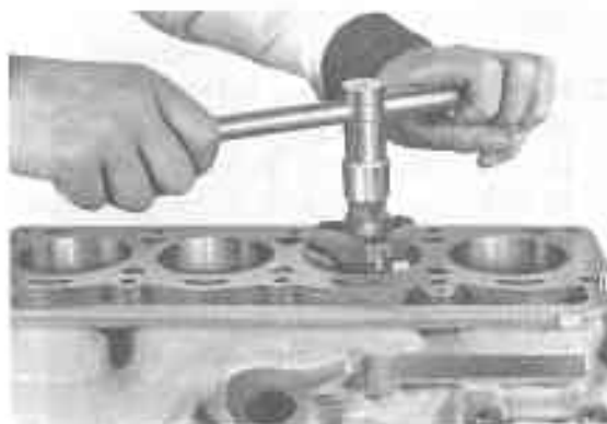
Fig. 3-32 Reaming Top of Bore V0725
