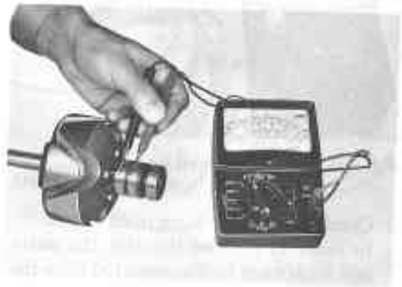
Fig. 8-13 Testing Rotor Coil for Open & Short Circuit
