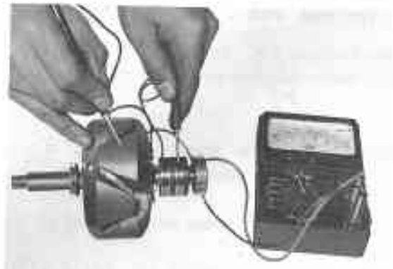
Fig. 8-14 Testing Rotor Coil for Ground
