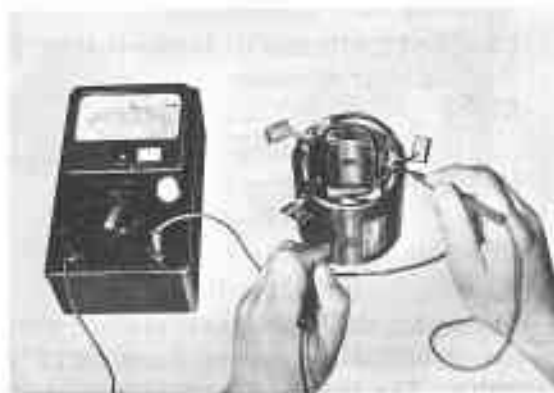
Fig. 9-14 Testing Field Coil for Ground
