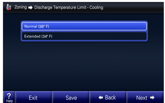
Discharge Temperature Limit Table
