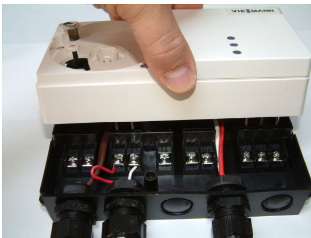
Fig. 5 Input Module with the module pulled off from its sub-base
