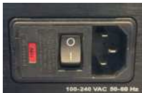
Step 5: Push the fuse holder cover in so that it is completely sealed.
