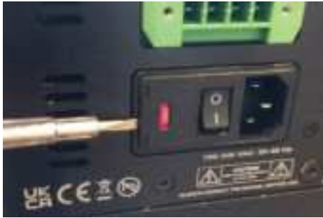
Step 1: Remove the fuse holder cover by using a flat head screwdriver as shown.
