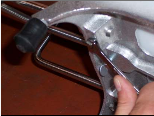
Figure 3. Pusher Head Adjustment Through the Blades.
