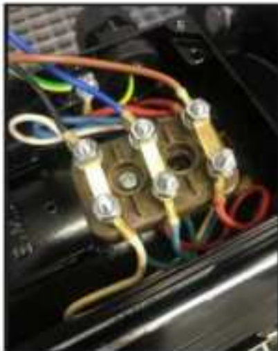
Fig.7 3-ph pump connection diagram
