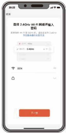
4. Select Wi-Fi Hotspot and enter your password The router network frequency must be 2.4G
